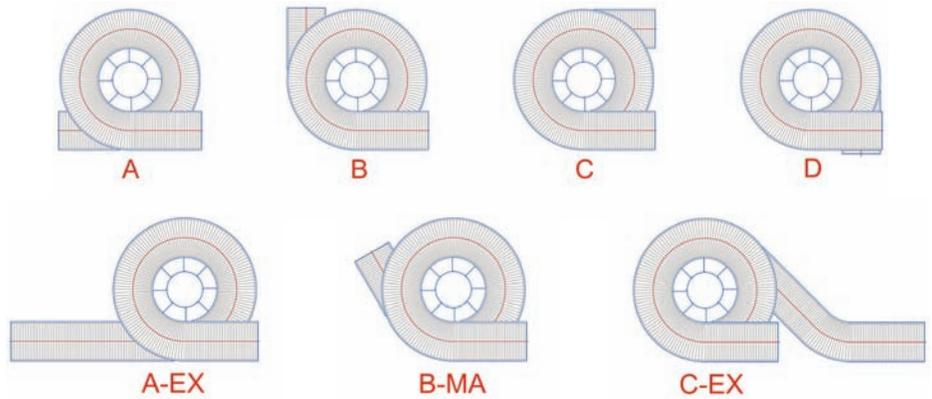
The position of the in feed tangent on up spirals and out feed tangent on down spirals can be customized to meet specific layout requirements. Samples are shown above (A-EX, B-MA and C-EX). A horizontal section is provided at in and out feed to assure smooth transition between conveyors. All Ryson Spirals are available in powder coated carbon steel, stainless steel, washdown, and freezer versions.
