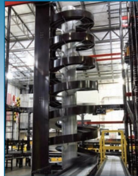
Ryson Spiral Conveyors need less floor space than conventional conveyors and are faster and more reliable than any elevator or lift. Ryson Spirals provide continuous vertical product flow and feature a small footprint, low maintenance and long life.
